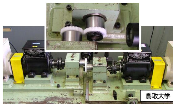
Fig.9 Photographs of test rig and test gears
